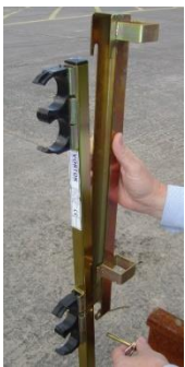
Figure 4 Light adaptor installation
